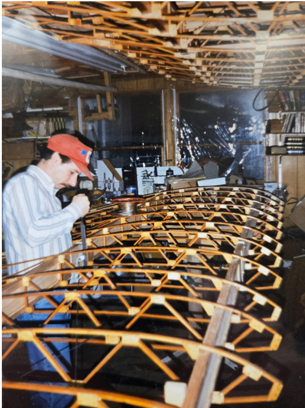
Therefore all 32 ribs can be made in one month. Craftsmanship, alignment and attention to detail are important here.
